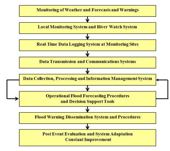
Figure 1: Elements of a Flood Warning System (Adapted from: Nemec 1986)
