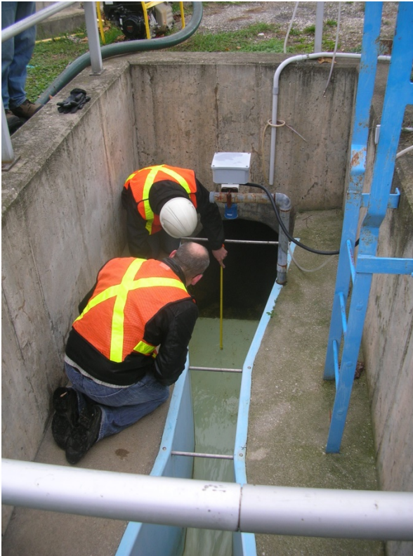
Figure 1: Photo (top) shows clarifier solids sampling at the Galt WWTP; photo (bottom) shows spot checking of the Parshall flume at the Paris WWTP
