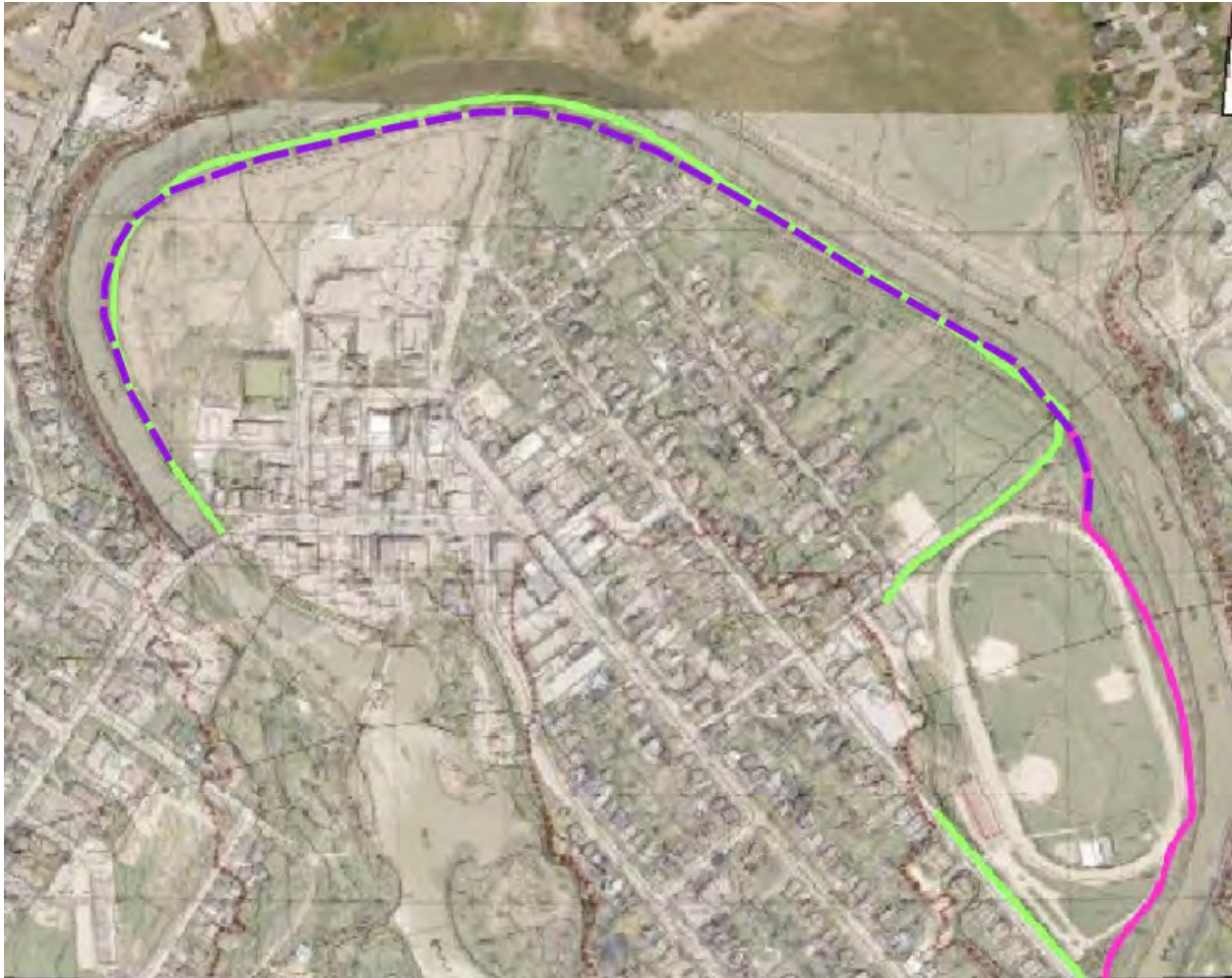
Graphic D Proposed Dike Improvements from Kilborn 1978 Option A (pink line), Option B (green line), Current Dike Alignment (purple, dashed line)
