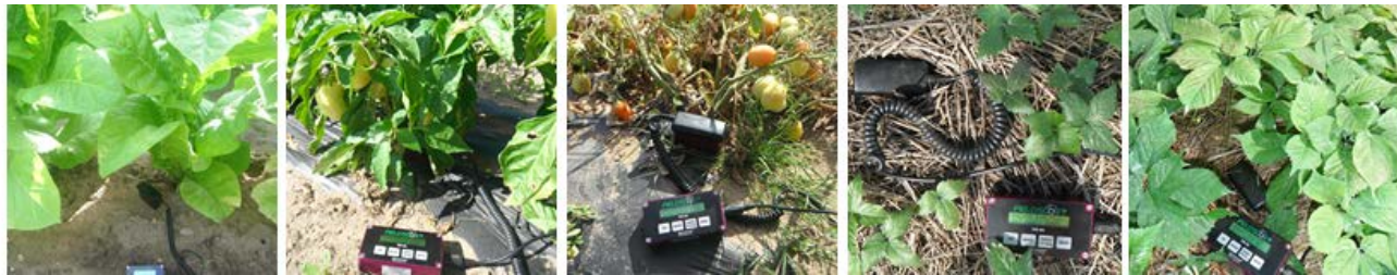
Figure 3: FieldScout TDR100 Soil Moisture Meter with 8” probes.
