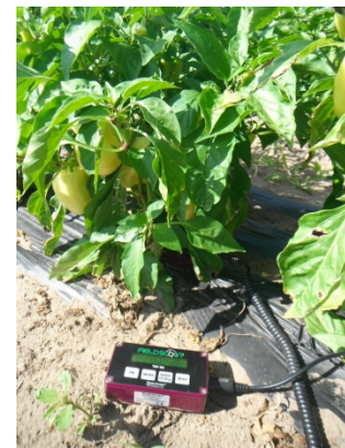
Figure 7: Reading soil moisture on peppers with plastic mulch in Brant County.
