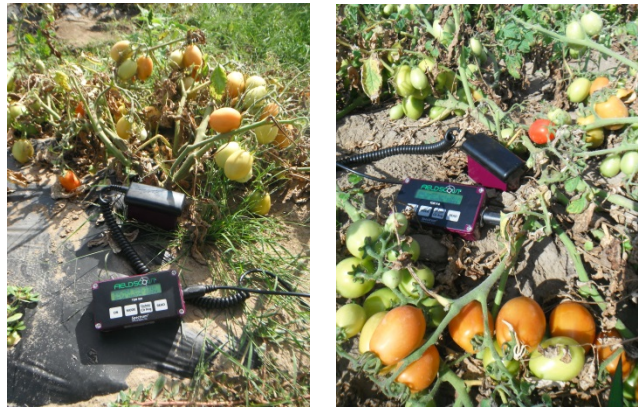
Figure 6: Reading the soil moisture on tomatoes with plastic mulch (on left) and without (on right) in Brant County.
