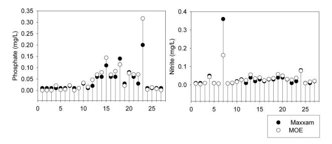
Figure A-3: Phosphate and nitrite concentrations analyzed by Maxxam (closed circles) and MOE (open circles) in 27 duplicate water samples.
