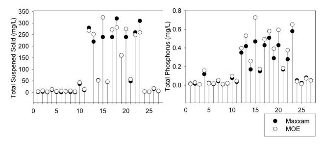
Figure A-4: Total suspended solid and total phosphorus concentrations analyzed by Maxxam (closed circles) and MOE (open circles) in 27 duplicate water samples.
