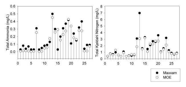
Figure A-2: Total ammonia and total Kjeldahl nitrogen concentrations analyzed by Maxxam (closed circles) and MOE (open circles) in 27 duplicate water samples.
