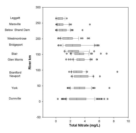
Figure 8-2: Box and whisker plots illustrating the range of total nitrate concentrations at sampling sites along the Grand River from the headwaters near Leggatt to Dunnville, near the mouth (2003-2008).
