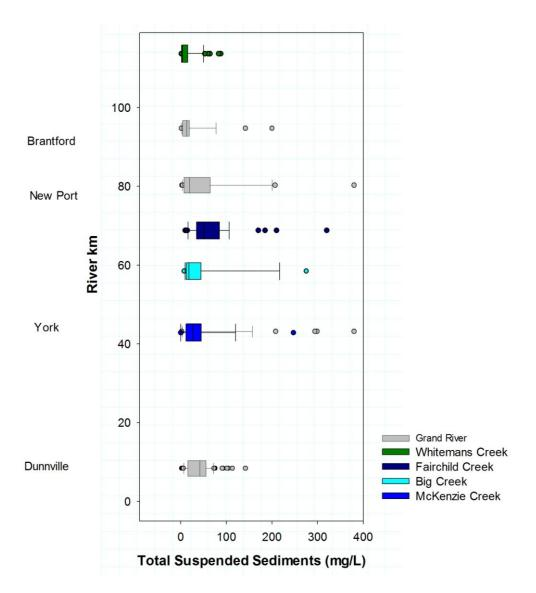
Figure 7- 10. Box and whisker plots illustrating the range of summer (June-September) total suspended sediment concentrations at water quality monitoring sites in the southern Grand River subbasin.
