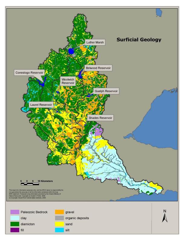
Figure 1-3: The surficial geology of the Grand River Watershed including the seven multipurpose reservoirs. Surficial geology is based on Quaternary and Pleistocene geology maps by the Ontario Geological Survey.
