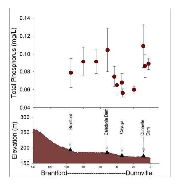
Figure B - 7 The average summer phosphorus levels (dot) and range (maximum and minimum) in the Grand River between Brantford and the Dunnville Dam. The bottom figure illustrates the elevation profile of the southern Grand River with the locations of on-line dams.
