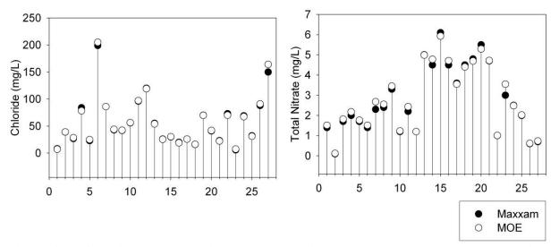
Figure A-1: Chloride and total nitrate concentrations analyzed by Maxxam (closed circles) and MOE (open circles) in 27 duplicate water samples.
