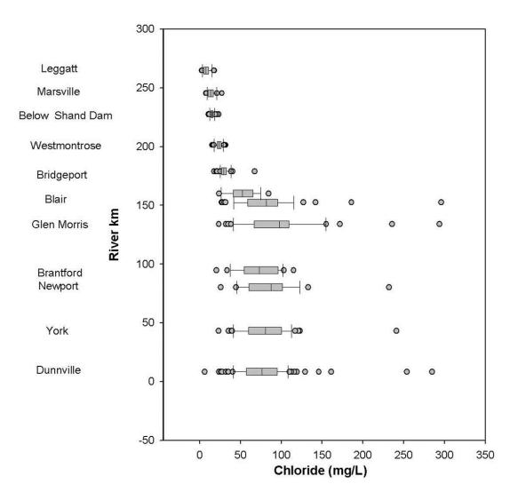
Figure 8-1: Box and whisker plots illustrating the range of chloride concentrations at sampling sites along the Grand River from the headwaters near Leggatt to Dunnville, near the mouth (2003-2008).
