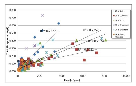
Figure B - 2. Relationship between total phosphorus (mg/L) and river flow ( $m^3$ /sec) at select locations on the Grand River. In general, the  $R^2$  values illustrates a stronger relationship between total phosphorus concentrations and flow.
