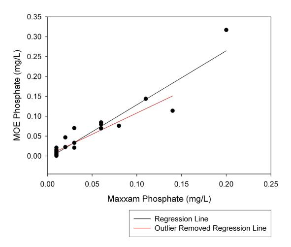
Figure A-6: The phosphate concentration measured by the MOE laboratory plotted against the phosphate concentration measured by the Maxxam laboratory.
