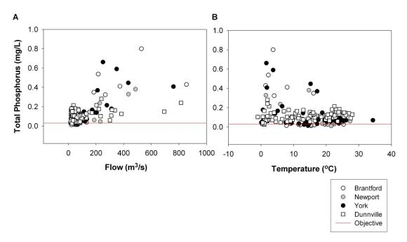
Figure 7-8: Total phosphorus concentrations in the southern Grand River subbasin relative to sampled flow (A) and field temperature (B).
