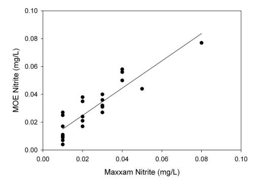
Figure A-5: The nitrite concentration measured by the MOW laboratory plotted against the concentration measured by the Maxxam laboratory.
