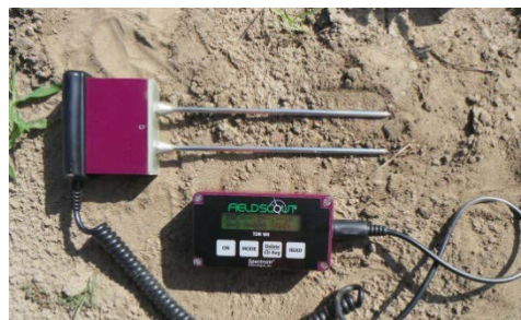
Figure 3: FieldScout TDR100 Soil Moisture Meter with 8” probes.
