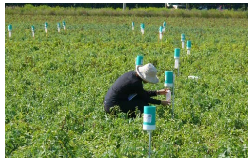
Figure 2: Gathering the volume of water collected in the "IrriGauges" after the centre pivot (Image 1) passed over them.
