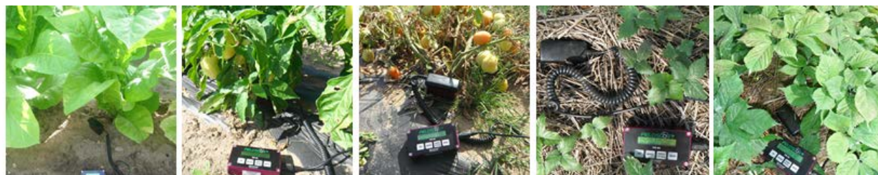
Figure 3: FieldScout TDR100 Soil Moisture Meter with 8” probes.
