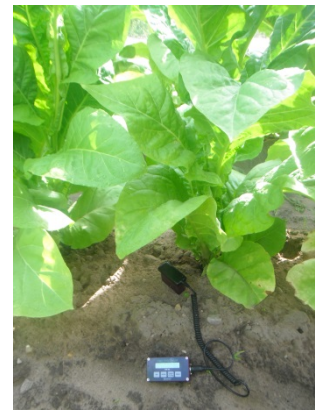
Figure 5: Reading the soil moisture on a tobacco plant in Oxford County.
