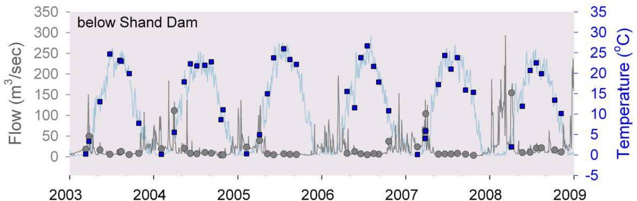
**Figure 6-3: Daily average flow (grey line) and temperature (blue boxes) sampled below Shand Dam relative to the flow timeseries of the West Montrose flow gauge and Bridgeport temperature monitoring site between 2003 and 2008.**
