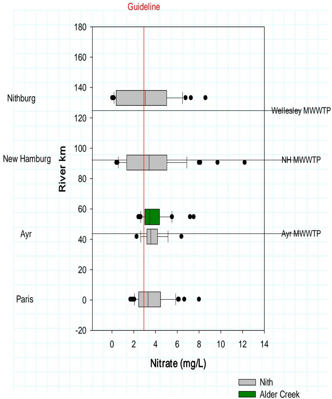
**Figure 5-5: Box and whisker plots illustrating the range of total nitrate concentrations (mg/L) at water quality monitoring sites in the Nith River subbasin between 2003 and 2008.**
