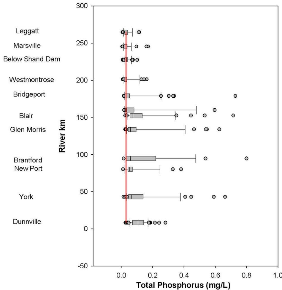
**Figure 8-3: Box and whisker plots illustrating the range of total phosphorus concentrations at sampling sites along the Grand River from the headwaters near Leggatt to Dunnville (2003-2008).**
