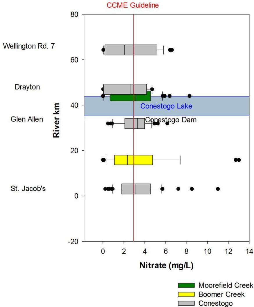
**Figure 3-7: Box and whisker plots illustrating the range of total nitrates (mg/L) in the Conestogo River subbasin, 2003-2008, relative to the federal environmental quality guideline of 2.93 mg/L (red line).**
