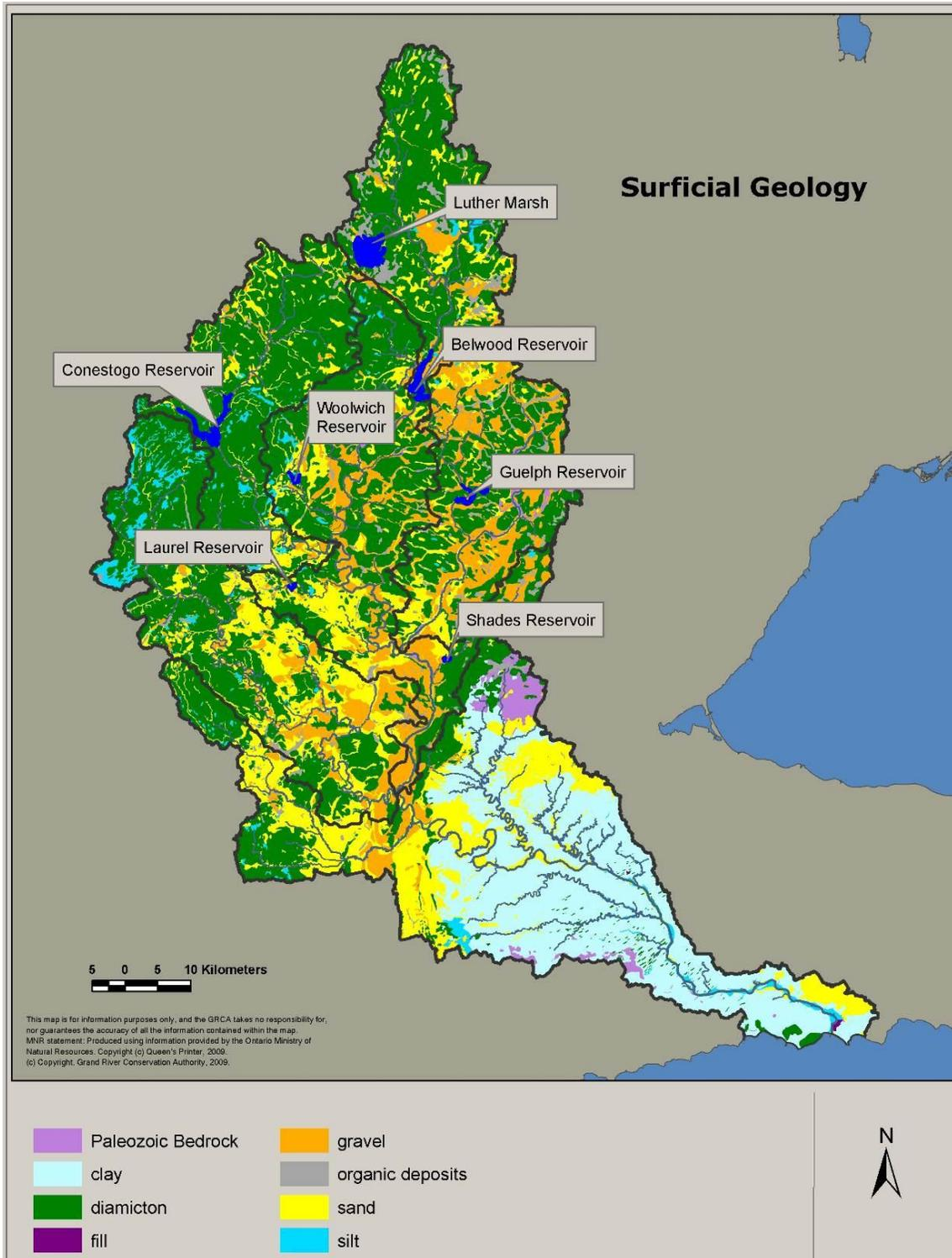
**Figure 1-3: The surficial geology of the Grand River Watershed including the seven multi-purpose reservoirs. Surficial geology is based on Quaternary and Pleistocene geology maps by the Ontario Geological Survey.**
