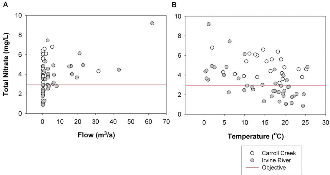
**Figure 6-18: Total nitrate concentrations (mg/L) in Carroll Creek and Irvine River in the central Grand River subbasin relative to sampled flow (A) and temperature (B).**
