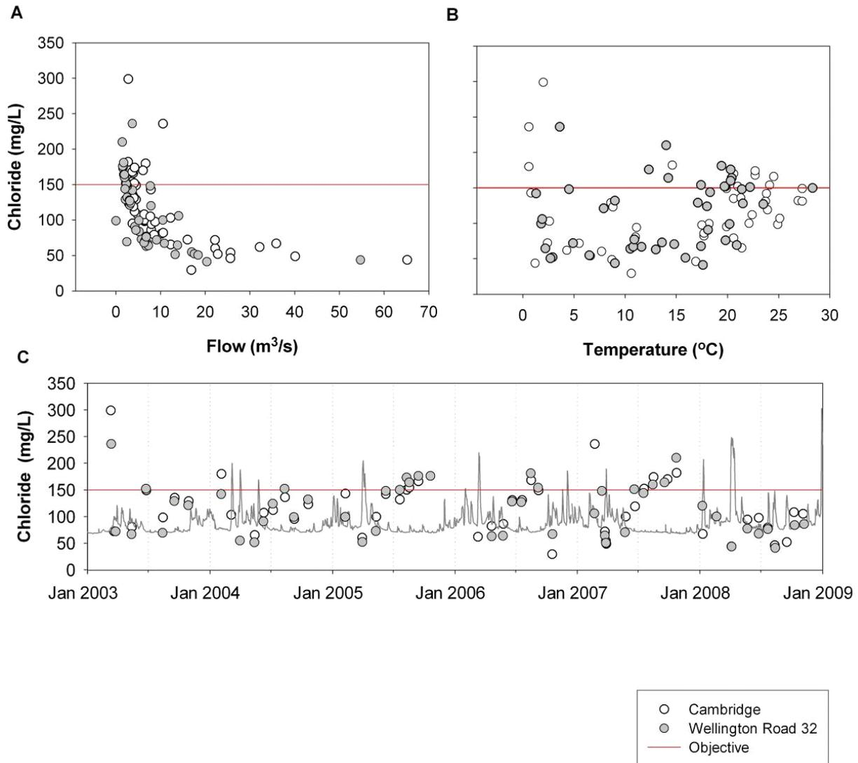
**Figure 4-8: Chloride concentrations in the Speed River at Wellington Rd. 32 and in Cambridge relative to flow (A), field temperature (B), and time (C).**
