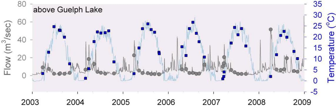
**Figure 4-3: Daily average flow (grey line) and temperature (blue boxes) sampled above Guelph Lake relative to the flow timeseries at the Hanlon flow gauge and Bridgeport temperature monitoring site between 2003 and 2008.**
