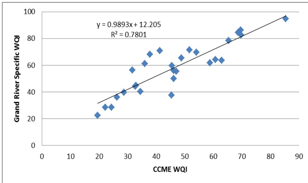
**Figure 8-5: The relationship between the Grand-River specific WQI using benchmarks specific to the Grand River and the CCME Nutrient WQI using provincial objectives.**
