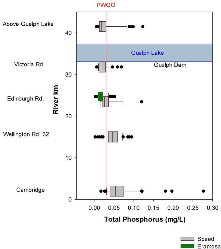
**Figure 4-15: Box and whisker plots illustrating the range of total phosphorus concentrations (mg/L) in the Speed River subbasin.**
