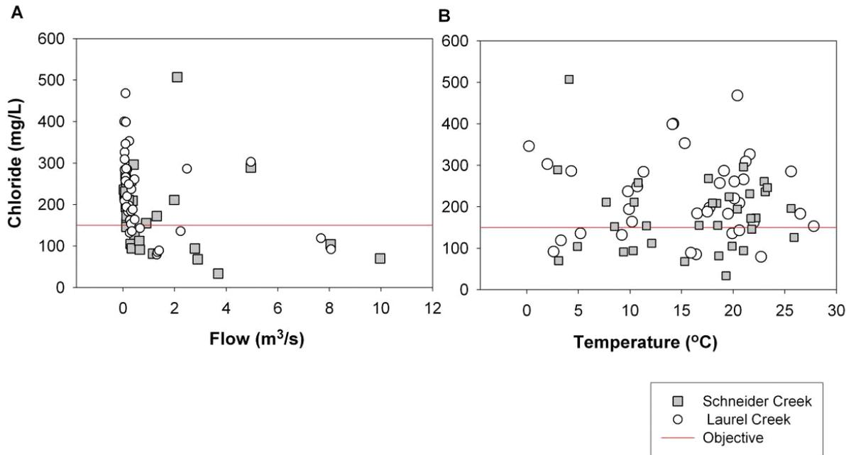
**Figure 6-10: Chloride concentrations (mg/L) in Schneider Creek and Laurel Creek relative to sampled flow (A) and temperature (B).**
