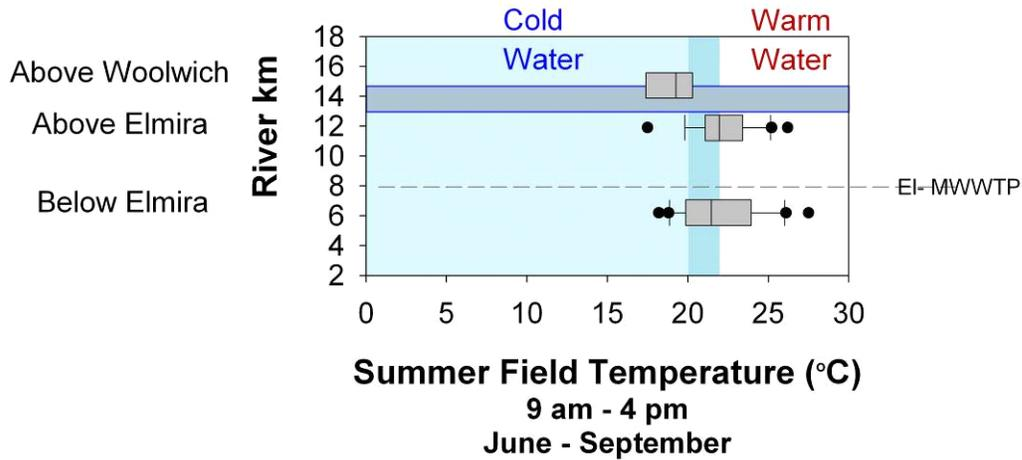
**Figure 6-5: Box and whisker plots illustrating the range of summer field daytime temperature on Canagagigue Creek, in the central Grand River subbasin.**
