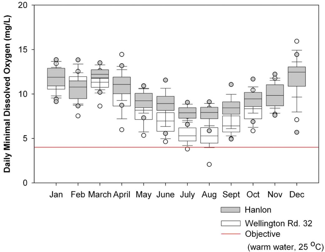
**Figure 4-5: Box plots showing the distribution of the daily minimum dissolved oxygen concentrations (mg/L) at the Edinburgh Road and Wellington Rd. 32 continuous water quality monitoring stations on the Speed River for data between 2003 and 2008. The red line represents the objective of 4 mg/L for warm water fishes.**
