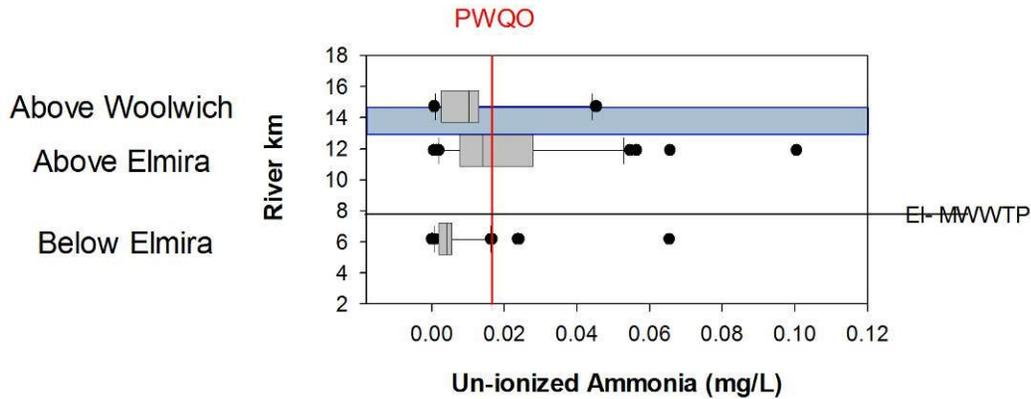
**Figure 6-15: Box and whisker plots illustrating the range of un-ionized ammonia (mg/L) in Canagagigue Creek in the central Grand River subbasin.**
