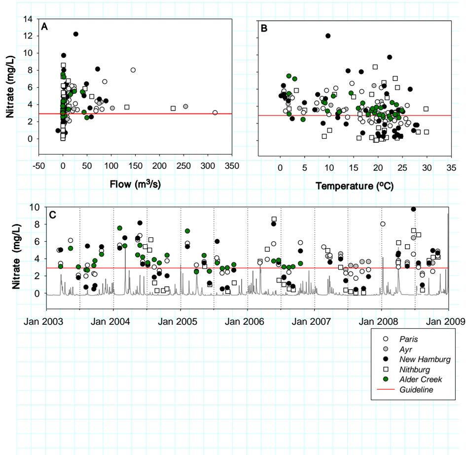
**Figure 5-6: Total nitrate concentrations (mg/L) at water quality monitoring sites in the Nith River subbasin relative to flow (A), stream temperature (B), the time (C).**
