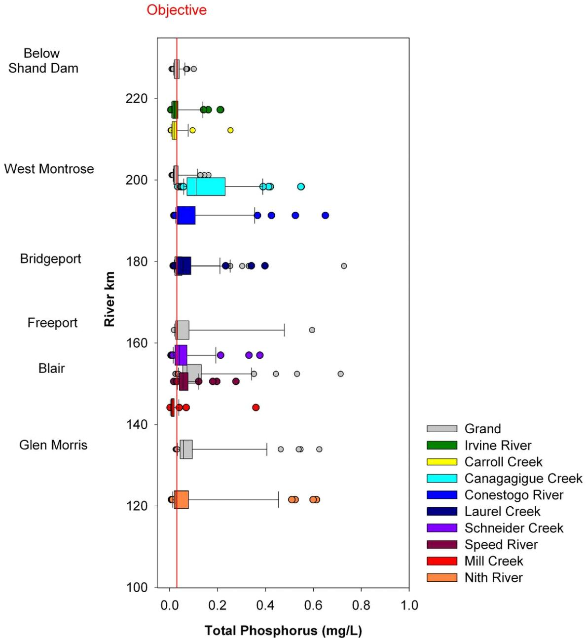
**Figure 6-21: Box and whisker plots illustrating the range of total phosphorus concentrations (mg/L) in the central Grand River subbasin.**
