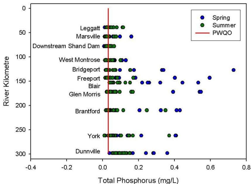
**Figure B - 1. Total phosphorus concentrations at monitoring sites from the headwater region (e.g. Leggatt) to Dunnville on the Grand River for Spring high flows (blue dots) and summer low flows (green dots). The red line is the Provincial Water Quality Objective. Data from the Provincial Water Quality Monitoring Network (2006-2010).**
