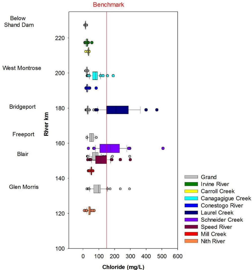
**Figure 6-9: Box and whisker plots illustrating the range of chloride concentrations (mg/L) observed at water quality monitoring sites in the central Grand River subbasin.**
