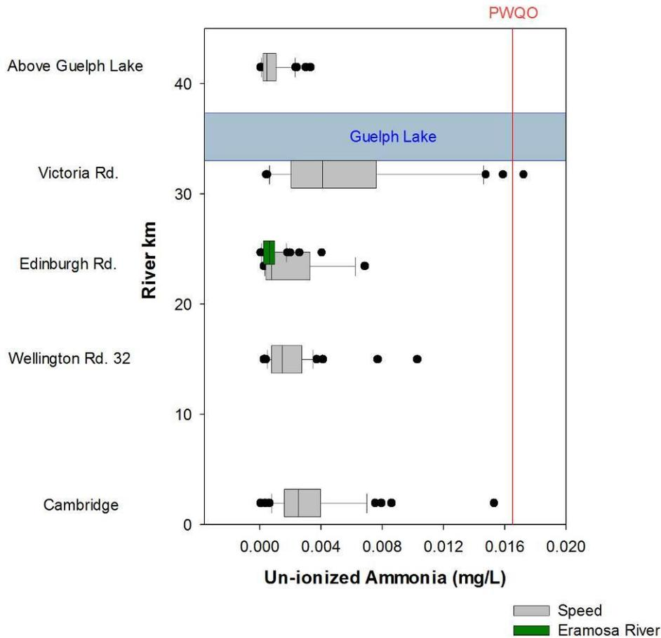
**Figure 4-10: Box and whisker plots illustrating the range of un-ionized ammonia concentrations (mg/L) at monitoring sites in the Speed River subbasin**
