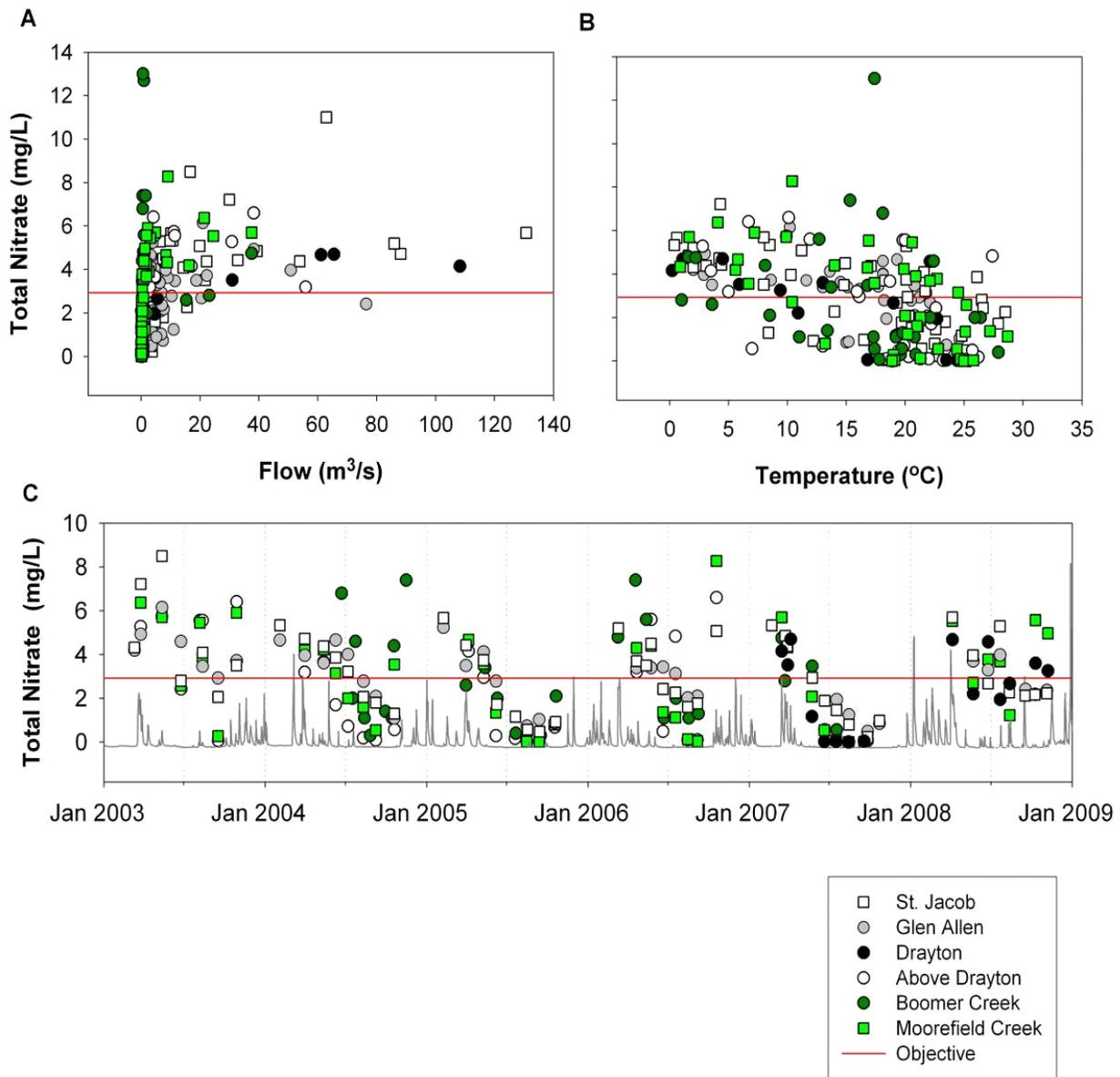
**Figure 3-8: Total nitrate concentrations (mg/L) at water quality monitoring sites in the Conestogo River subbasin relative to sampled flow (A), field temperature (B), and time (C).**
