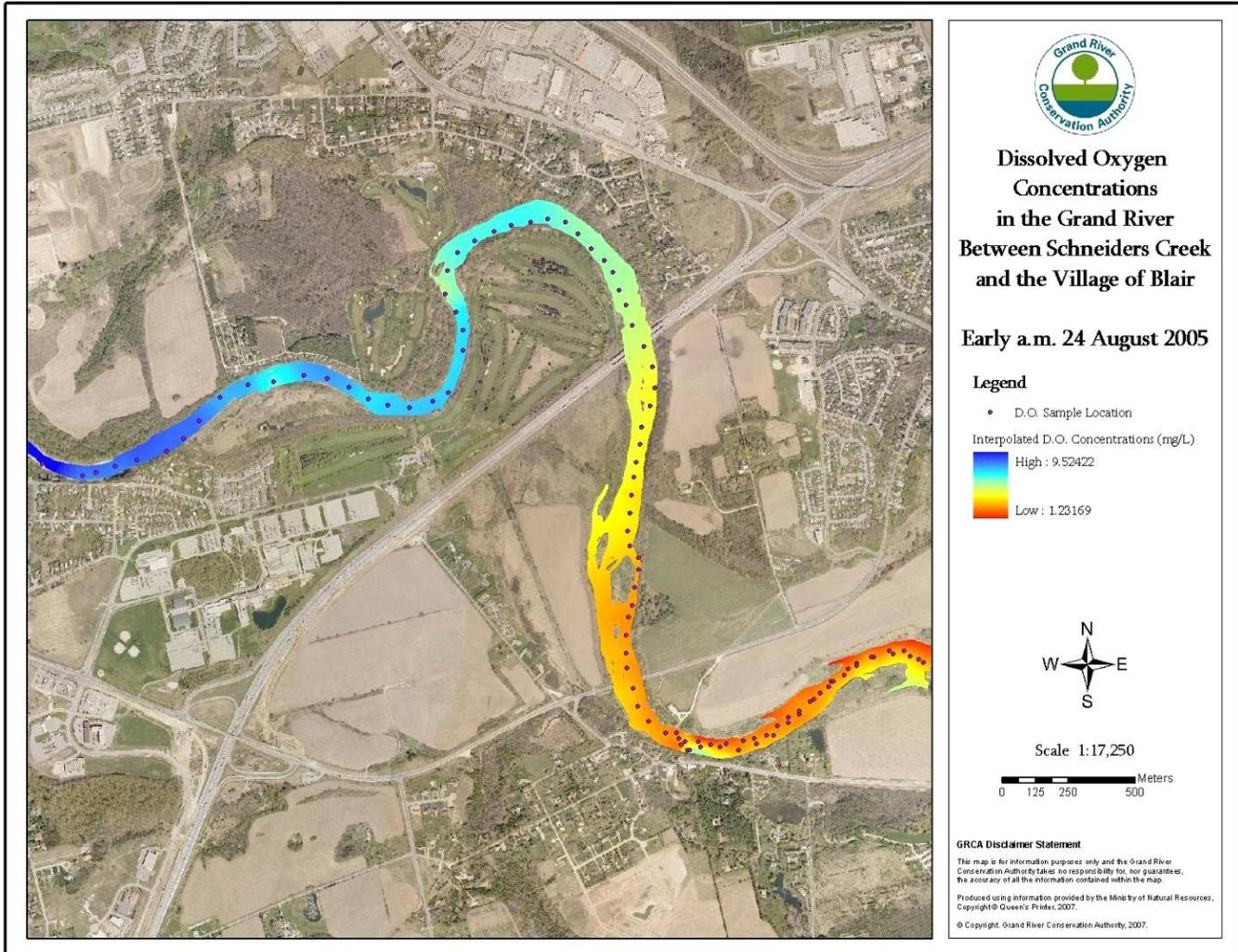
**Figure 6-8: Observed dissolved oxygen concentrations between Schneider Creek and Blair on the Grand River between 6 and 8 am on August 24th, 2005.**
