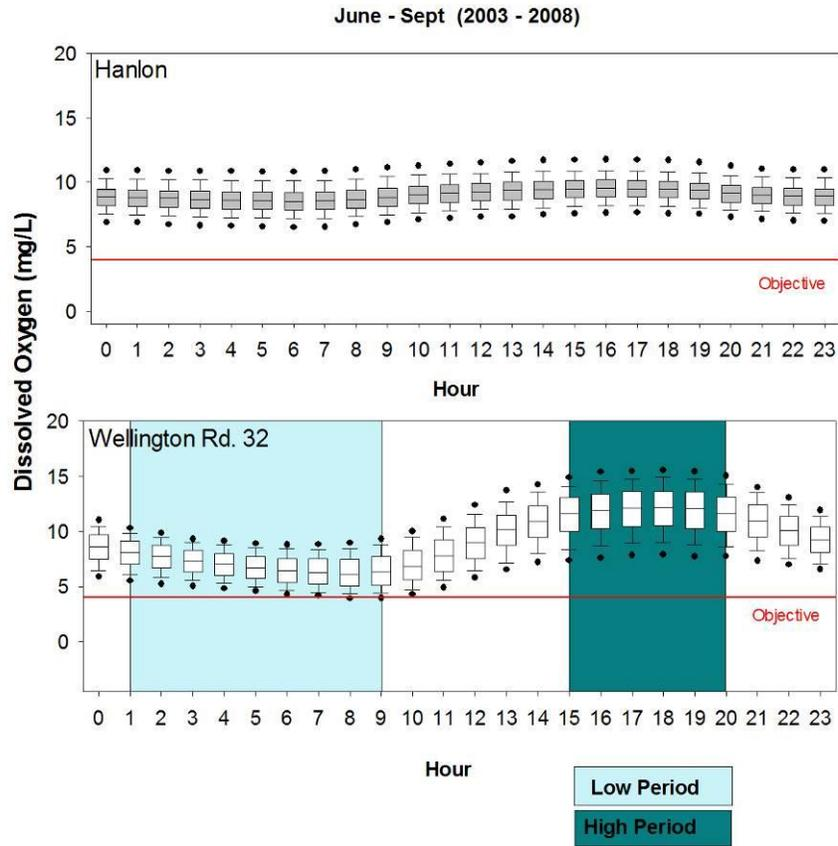
**Figure 4-6: Box plots showing the range and distribution of dissolved oxygen concentrations between June and September at two continuous monitoring stations on the Speed River. The red line represents the objective of 4 mg/L for warm water fishes.**
