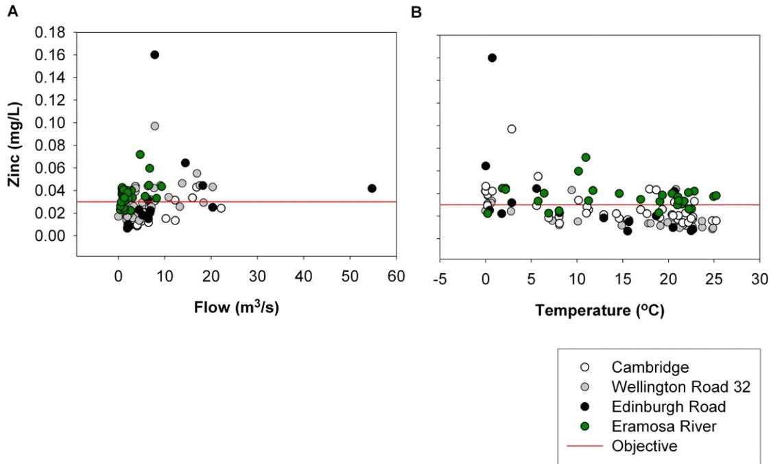
**Figure 4-20: Zinc concentrations (mg/L) in the Eramosa River and in the Speed River at Edinburgh Rd, Wellington Rd. 32, and Cambridge sites relative to sampled flow (A) and stream temperature (B).**
