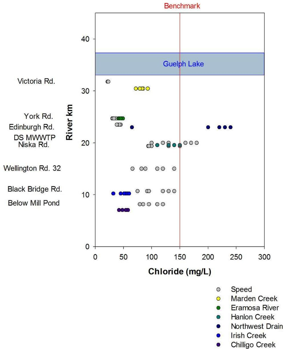
**Figure 4-9: Chloride concentrations (mg/L) in the Speed River and select tributaries arranged by river kilometre between July and August 2008.**
