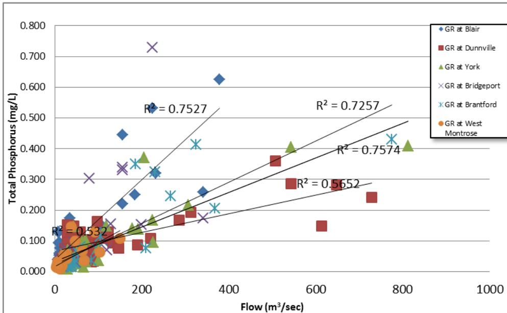
**Figure B - 2. Relationship between total phosphorus (mg/L) and river flow (m<sup>3</sup>/sec) at select locations on the Grand River. In general, the R<sup>2</sup> values illustrates a stronger relationship between total phosphorus concentrations and flow.**
