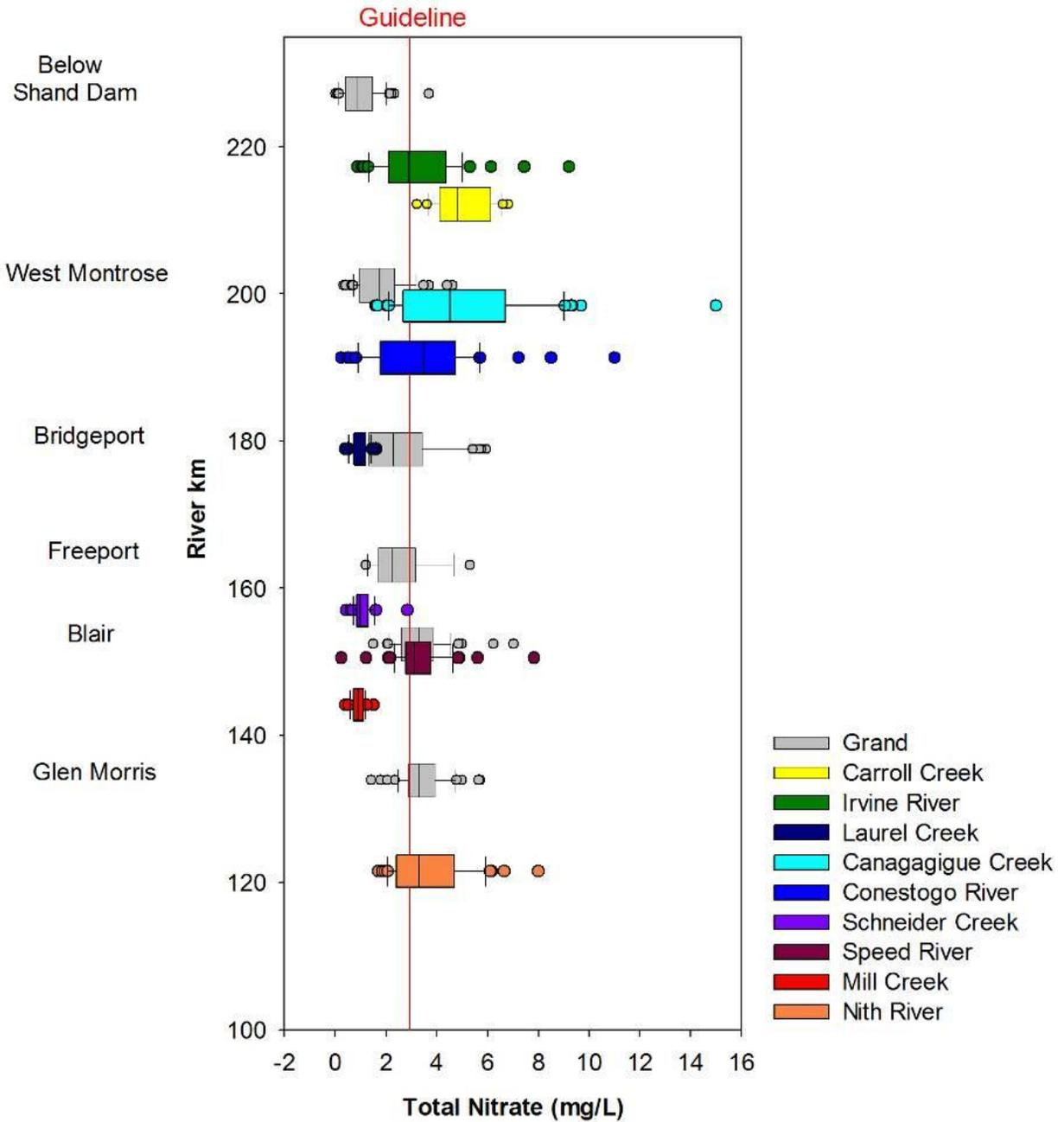
**Figure 6-16: Box and whisker plots illustrating the range of total nitrate concentrations (mg/L) in the central Grand River subbasin (2003 – 2008).**
