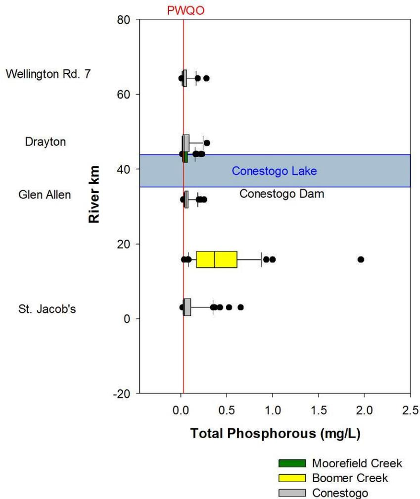
**Figure 3-9: Box and whisker plots illustrating the range of total phosphorus concentrations (mg/L) in the Conestogo River subbasin, data from 2003-2008, relative to the Provincial Water Quality Objective of 0.03 mg/L.**
