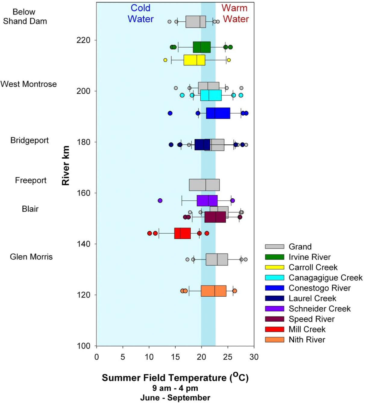
**Figure 6-4: Box and whisker plots illustrating the range of summer (June – September) daytime (9 am - 4 pm) field temperatures in the central Grand River subbasin.**
