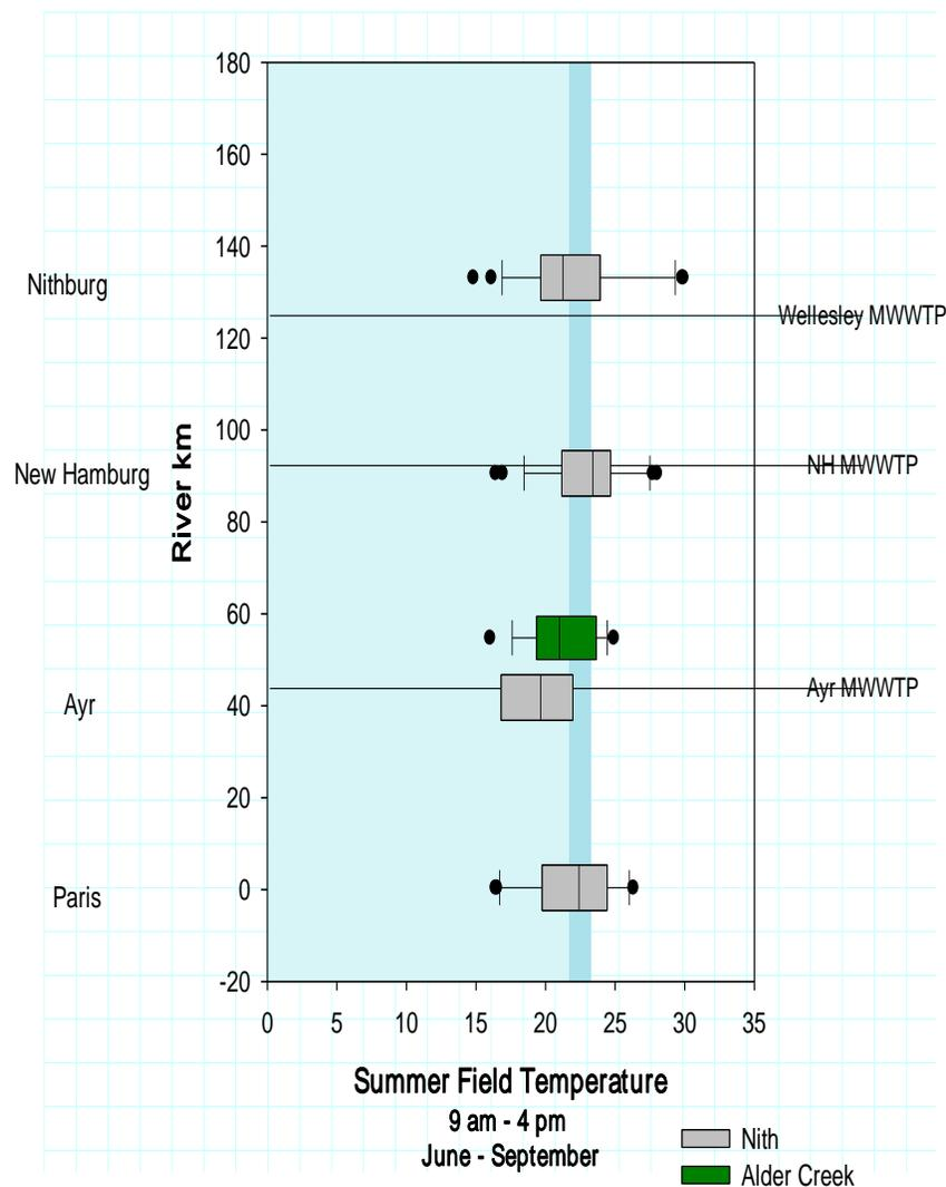
**Figure 5-4: Box and whisker plots illustrating the range of summer (June – September) daytime (9 am - 4 pm) field temperatures in the Nith River Watershed**
