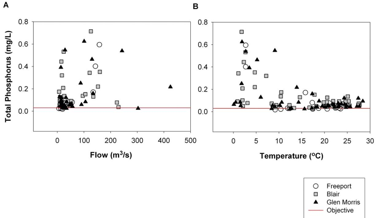
**Figure 6-22: Total phosphorus concentrations (mg/L) in the Grand River in the central Grand River subbasin relative to sampled flow (A) and temperature (B), 2003-2008.**
