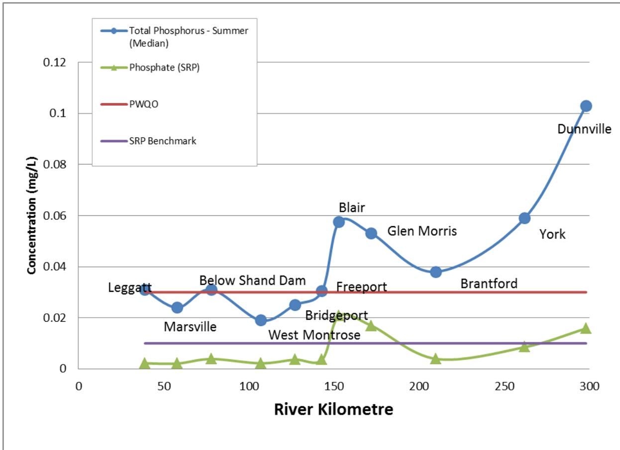
**Figure B - 6. Representative total phosphorus and soluble reactive phosphorus (a measure of biologically available phosphorus or phosphate) concentrations along the Grand River from the headwaters (Leggatt) to the mouth of the Grand River near Dunnville during low flow conditions (e.g. June – September). The red line is the Provincial Water Quality Objective of 0.030 mg/L.**
