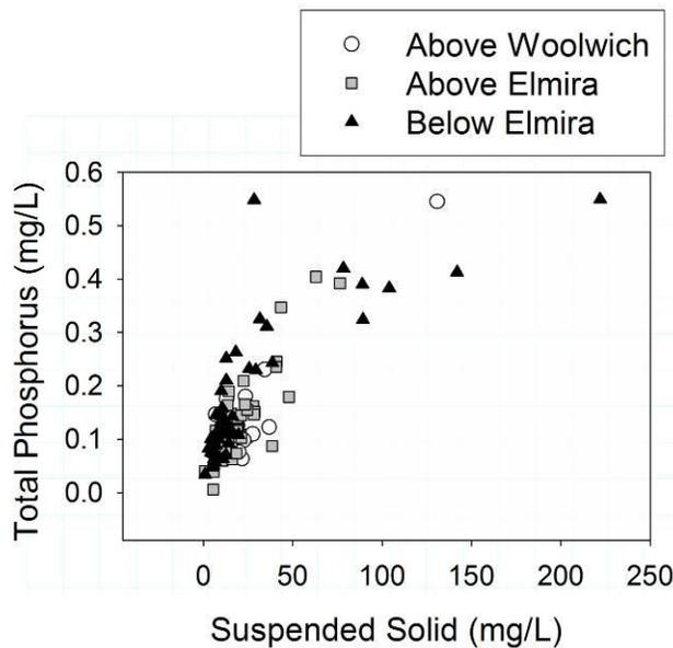
**Figure 6-27: Total phosphorus concentrations relative to suspended solids in Canagagigue Creek in the central Grand River subbasin**
