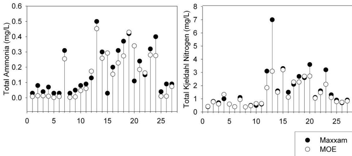
**Figure A-2: Total ammonia and total Kjeldahl nitrogen concentrations analyzed by Maxxam (closed circles) and MOE (open circles) in 27 duplicate water samples.**
