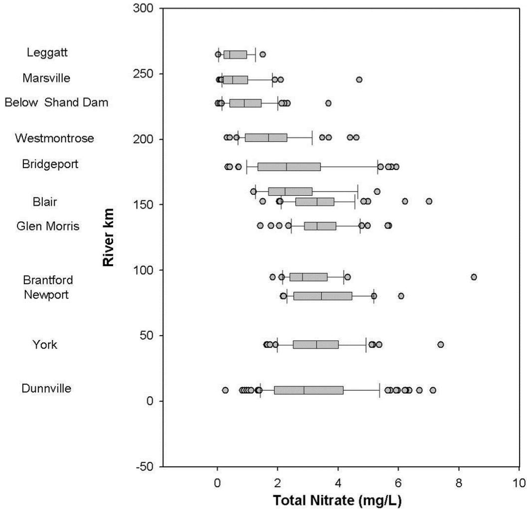
**Figure 8-2: Box and whisker plots illustrating the range of total nitrate concentrations at sampling sites along the Grand River from the headwaters near Leggatt to Dunnville, near the mouth (2003-2008).**
