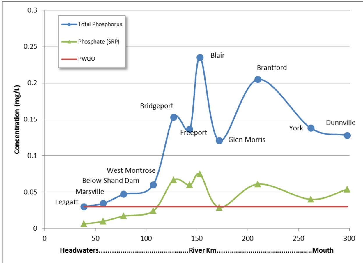
**Figure B - 5. Representative total phosphorus and soluble reactive phosphorus (a measure of biologically available phosphorus or phosphate) concentrations along the Grand River from the headwaters (Leggatt) to the mouth of the Grand River near Dunnville during spring (e.g. March/April) high flow conditions. The red line is the Provincial Water Quality Objective of 0.030 mg/L.**
