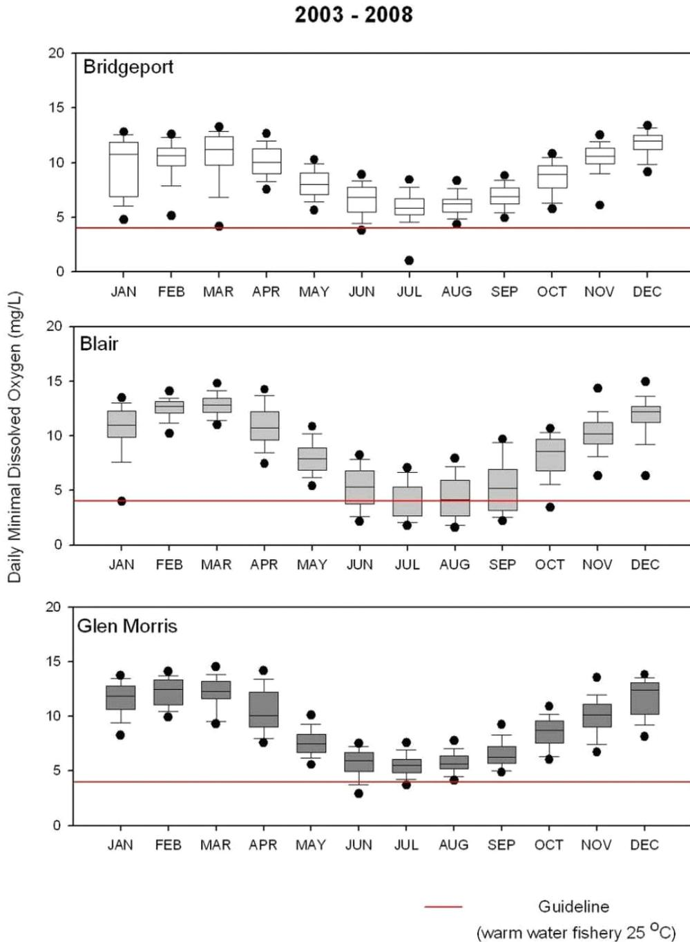
**Figure 6-6: Box and whisker plots illustrating the range of the daily minimum dissolved oxygen concentrations by month from the continuous monitoring records at Bridgeport (top), Blair (middle), and Glen Morris (bottom). The red line represents the PWQO of 4 mg/L for warm water fish.**
