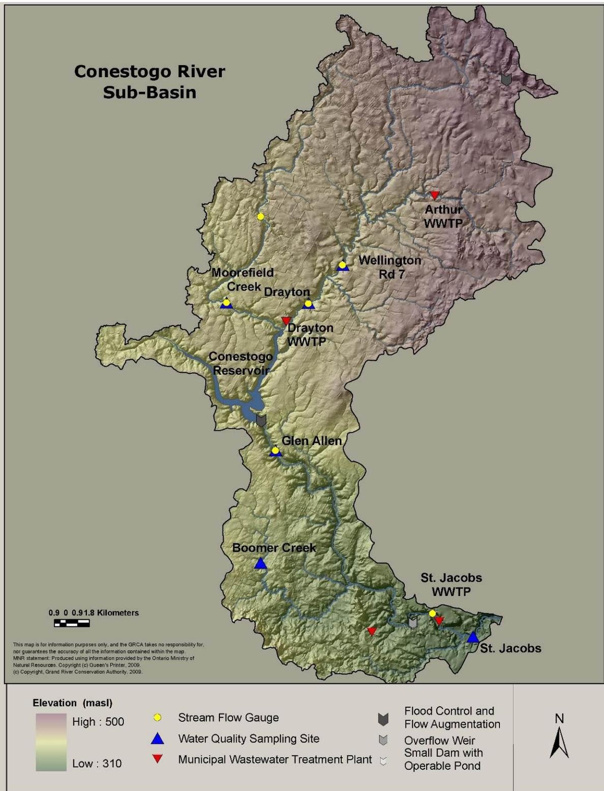
**Figure 3-1: The water quality sampling sites, flow gauge locations, and municipal wastewater treatment plants in the Conestogo River subbasin.**
