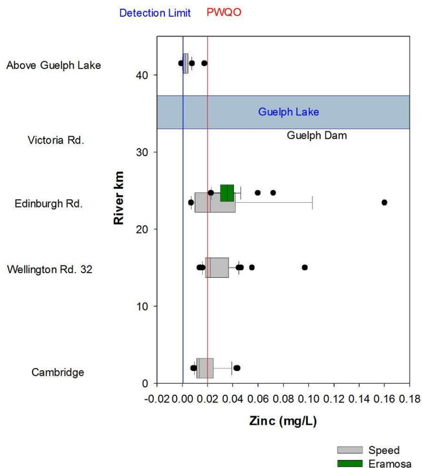
**Figure 4-19: Box and whisker plots showing the range of zinc concentrations (mg/L) in the Speed River subbasin**
