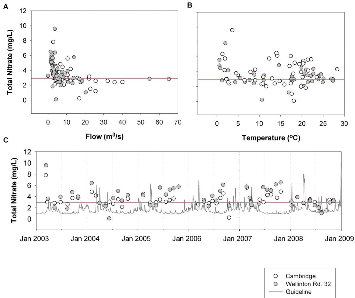
**Figure 4-13: Total nitrate concentrations (mg/L) at Wellington Rd. 32 and Cambridge in the Speed River relative to sampled flow (A), field temperature (B), and time (C).**
