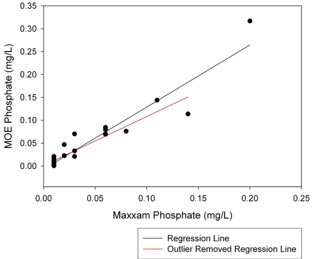
**Figure A-6: The phosphate concentration measured by the MOE laboratory plotted against the phosphate concentration measured by the Maxxam laboratory.**
