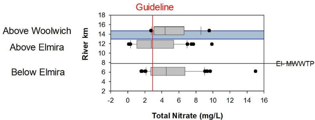
**Figure 6-19: Box and whisker plots illustrating the range of total nitrate concentrations (mg/L) (2003 – 2008) in the Canagagigue Creek, located in the central Grand River subbasin.**
