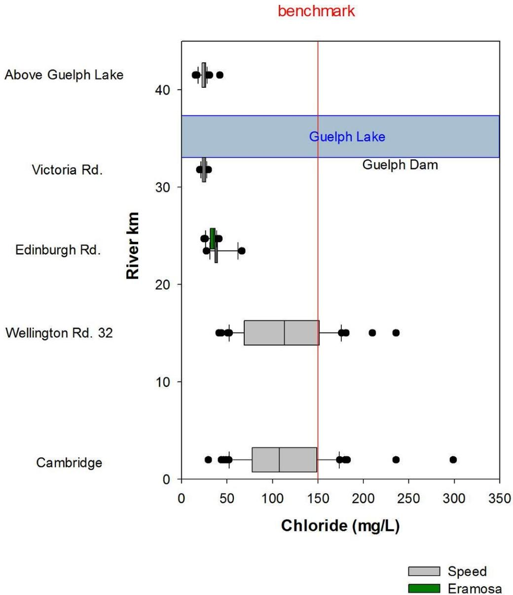
**Figure 4-7: Box and whisker plots showing the range of chloride concentrations at monitoring sites in the Speed - Eramosa river subbasin between 2003 and 2008.**
