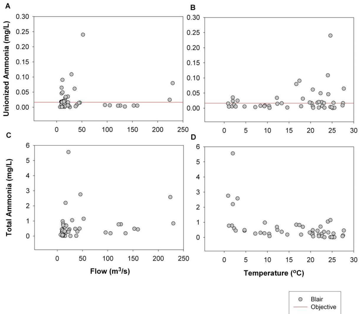
**Figure 6-14: Un-ionized ammonia (A) relative to flow (A) and temperature (B) and total ammonia concentrations relative to flow (C) and temperature (D) at Blair.**
