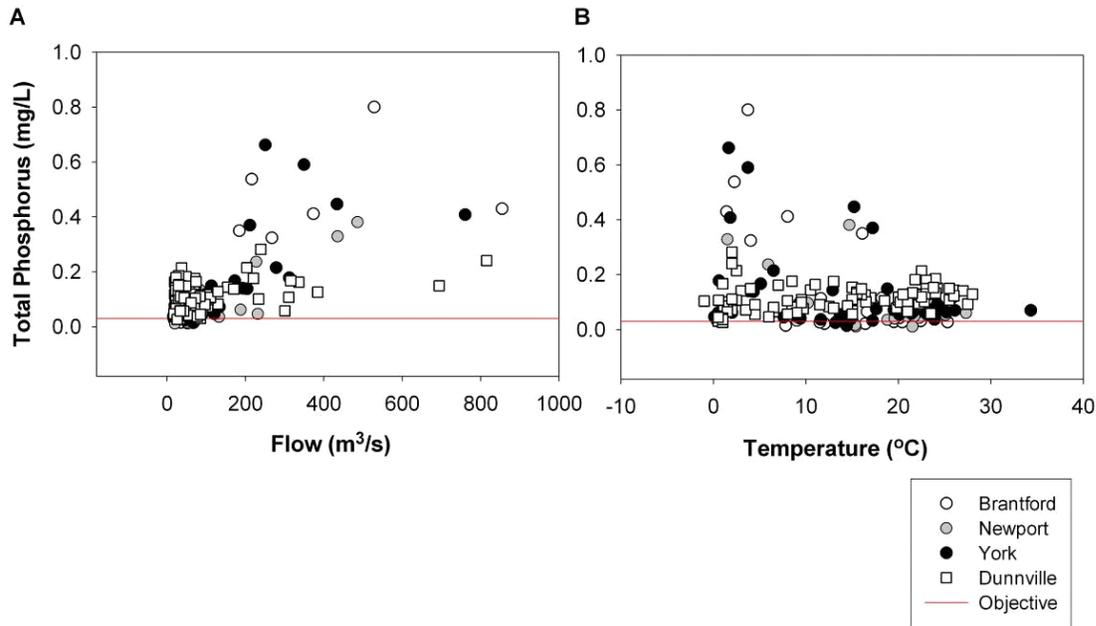
**Figure 7-8: Total phosphorus concentrations in the southern Grand River subbasin relative to sampled flow (A) and field temperature (B).**
