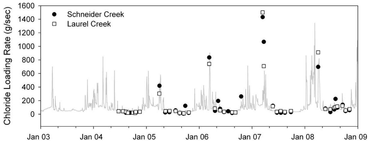
**Figure 6-11: The chloride loading (g/sec) rate in Schneider Creek and Laurel Creek in comparison with the hydrograph**
