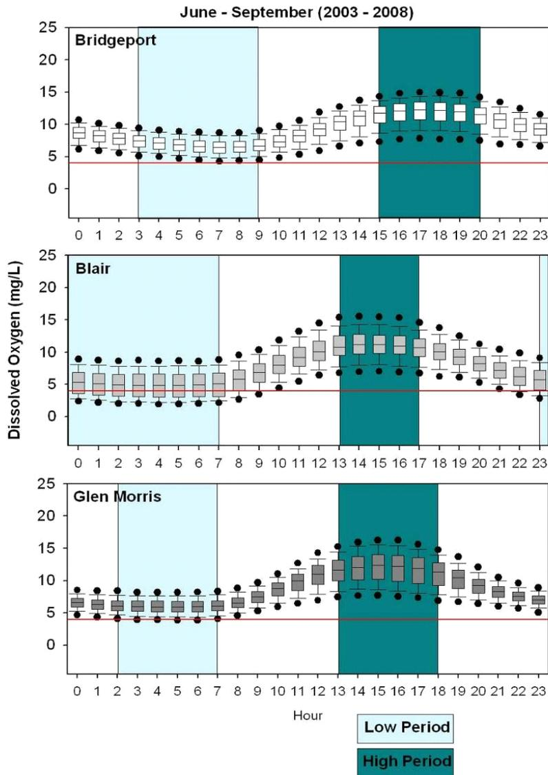
**Figure 6-7: Box and whisker plots illustrating the range of the hourly dissolve oxygen concentrations (mg/L) at Bridgeport (top), Blair (middle), and Glen Morris (bottom) between June and September. The red line represents the PWQO of 4 mg/L.**
