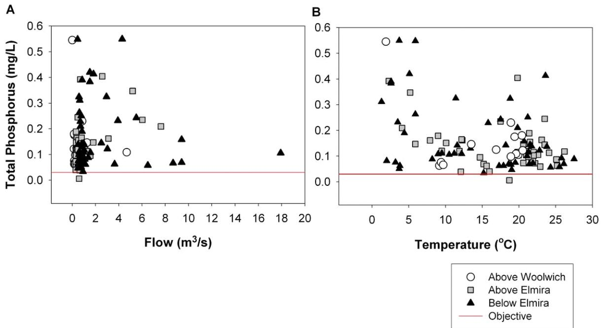
**Figure 6-24: Total phosphorus concentrations (mg/L) in Canagagigue Creek (2003 – 2008) in the central Grand River subbasin relative to sampled flow (A) and temperature (B).**
