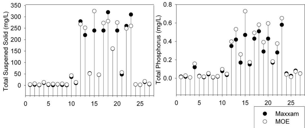
**Figure A-4: Total suspended solid and total phosphorus concentrations analyzed by Maxxam (closed circles) and MOE (open circles) in 27 duplicate water samples.**
