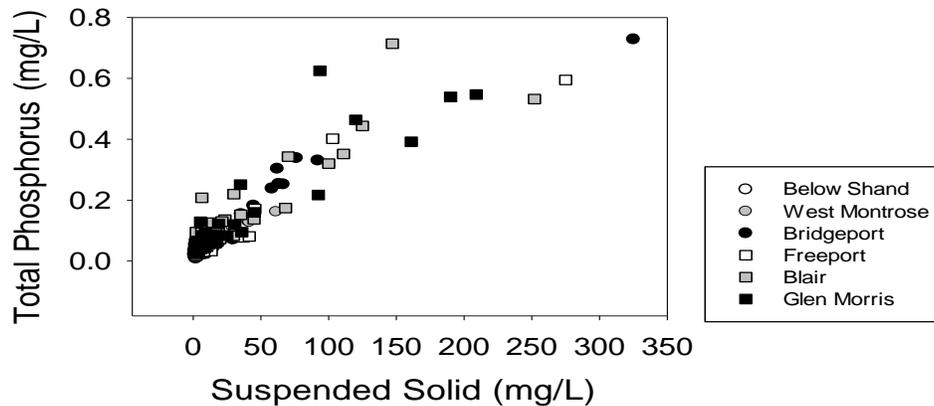
**Figure 6-25: Total phosphorus concentrations relative to suspended solids concentrations at sampling sites in the central Grand River subbasin.**
