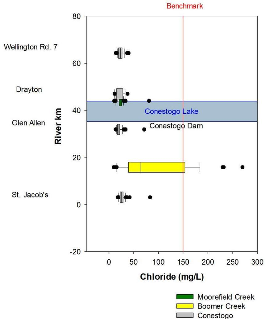
**Figure 3-5: Box and whisker plots illustrating the range of chloride concentrations (mg/L) in the Conestogo River subbasin, 2003-2008, relative to the benchmark of 150 mg/L (red line).**
