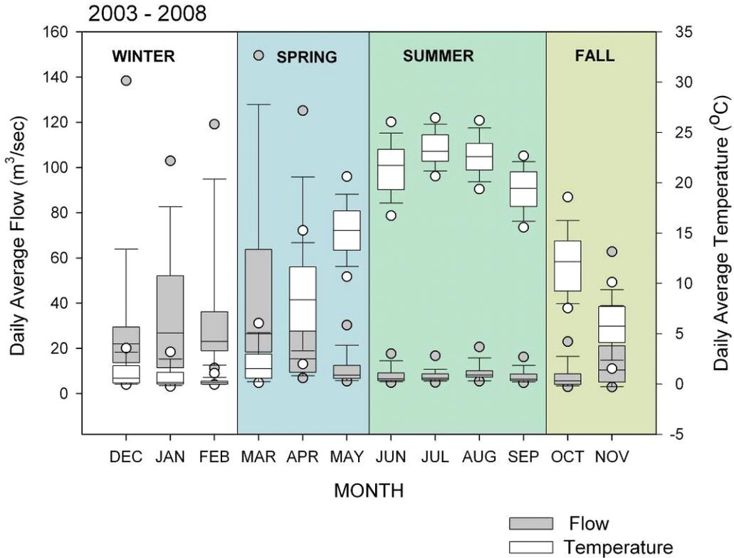
**Figure 1-17: Monthly average temperature and flow in the Grand River at the continuous monitoring station at Bridgeport (2003-2008).**
