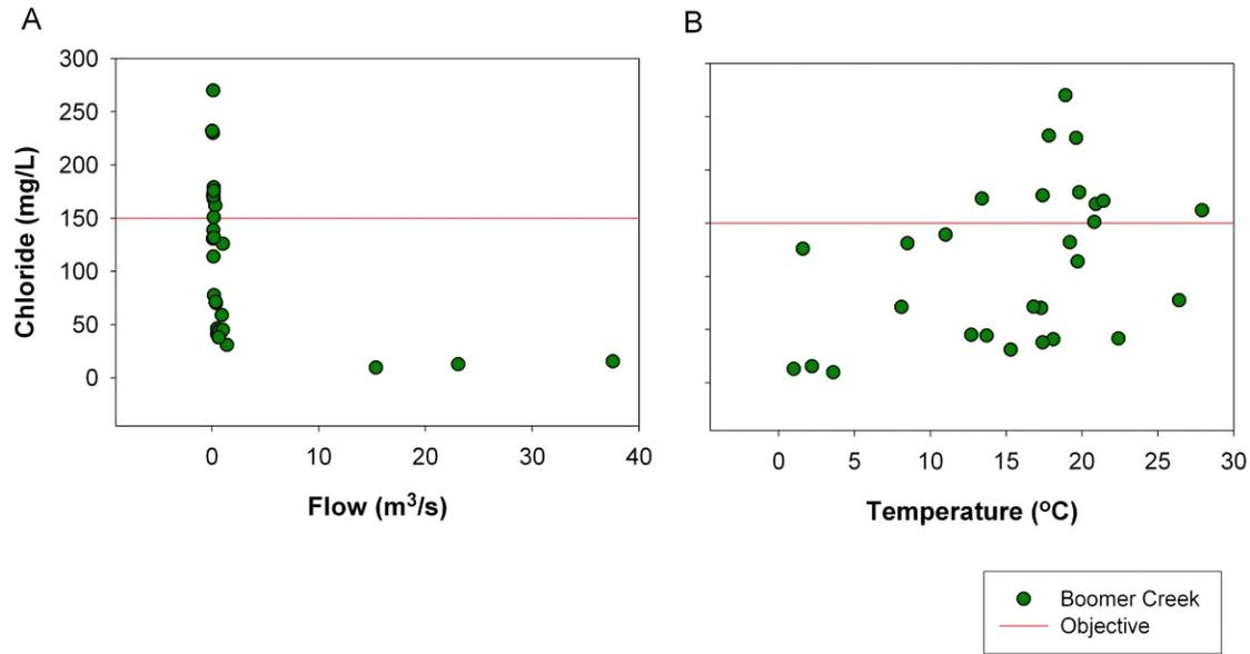
**Figure 3-6: Chloride concentrations in Boomer Creek relative to flow (A) and field temperature (B).**
