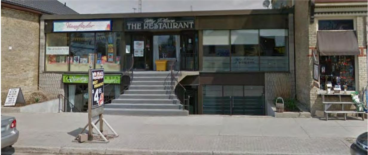
**Graphic M** Special Case: Set First-floor Elevation as Mean Ground Surface Minus Number of Steps
