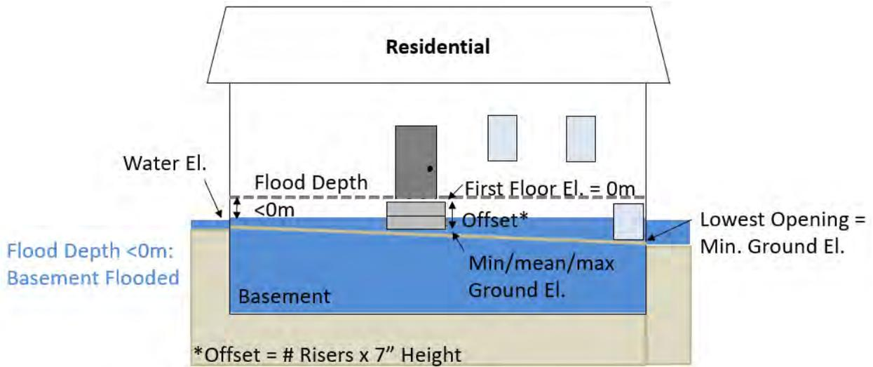
**Graphic S** Schematic of Residential Building with Basement and Flooding Below First Floor
