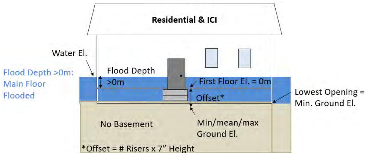
**Graphic T** Schematic of Residential/Industrial, Commercial, or Institutional Building without Basement and Flooding Above First Floor
