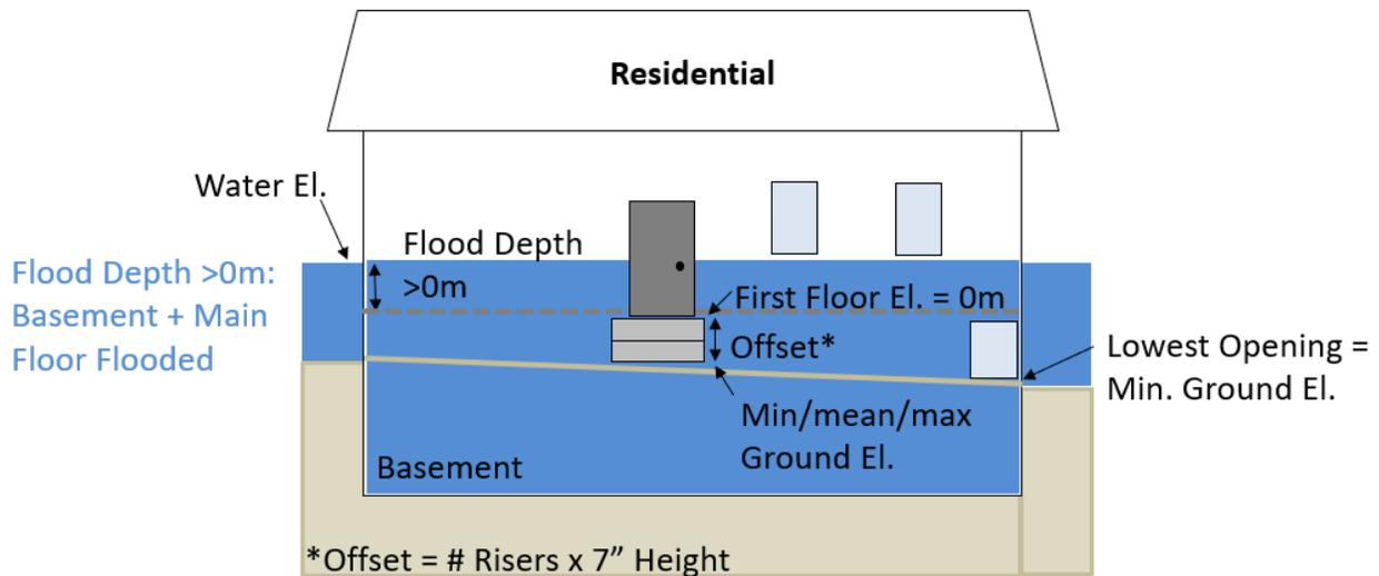
**Graphic R Schematic of Residential Building with Basement and Flooding Above First Floor**
