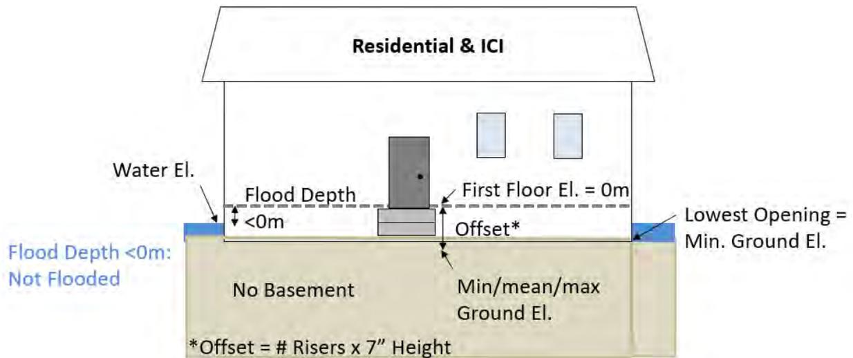
**Graphic U** Schematic of Residential/Industrial, Commercial, or Institutional Building without Basement and Flooding Below First Floor
