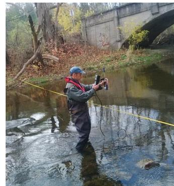
*Collecting river flow data allows engineers to calibrate flood forecast models*
