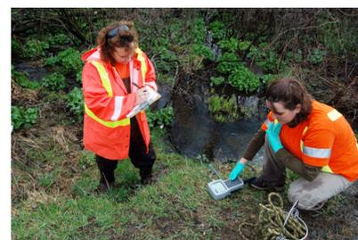
*Collecting stream water quality samples help to gauge the health of the stream*
